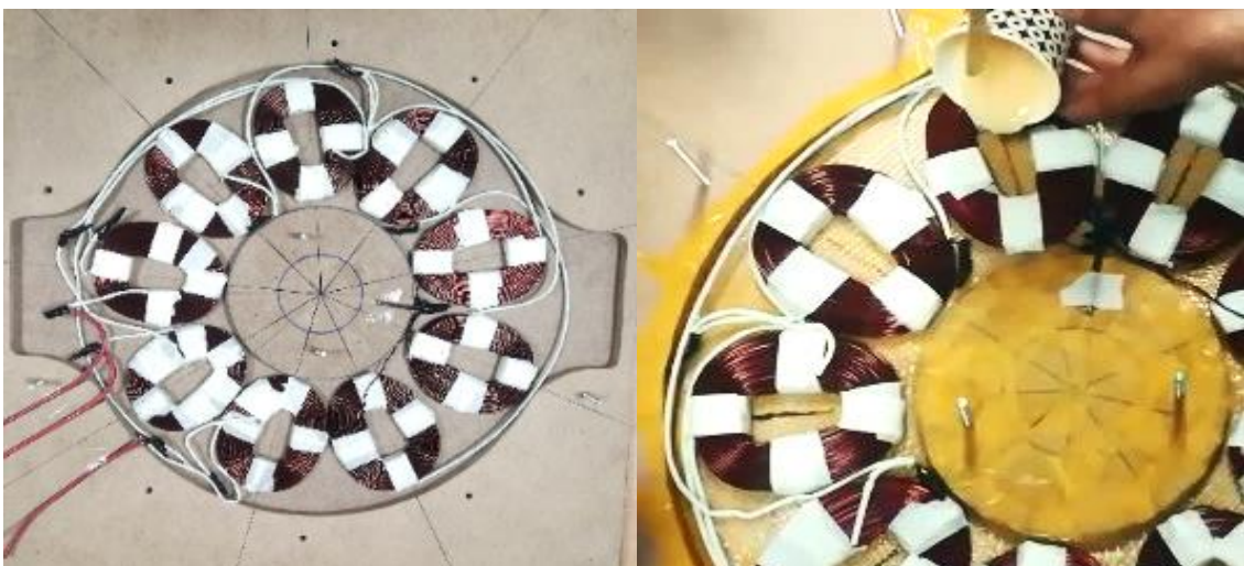
Figure 10. Coil Adjustment & Epoxy Filling
