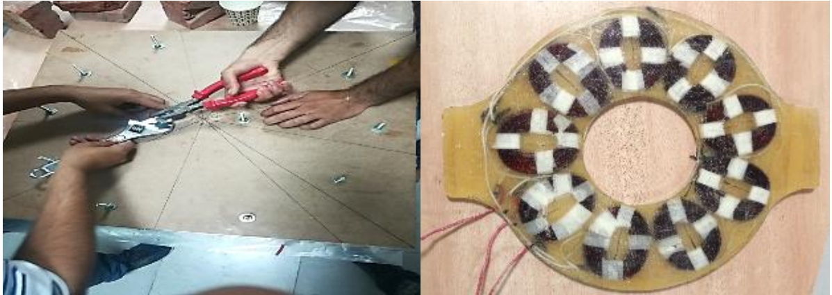
Figure 11. Stator Coil Ring and Mold
