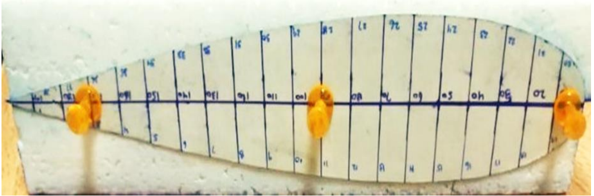
Figure 8. The Chord Attached to the Thermocol Sheet
